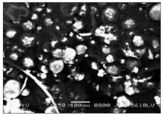
Fig. 1: SEM photograph of chitosan microspheres. SEM photograph of microspheres was recorded at 150X magnification to characterize shape and surface properties of the microspheres.
