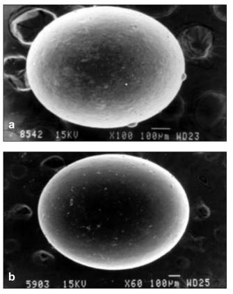
Fig. 1: SEM Photomicrographs. Photomicroghaphs of Cellulose acetate cores (a) and Eudragit S microcapsules (b) as revealed by scanning electron microscopy.
