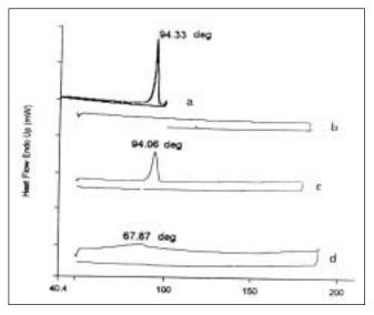
Fig. 3: Differential scanning calorimetric scan. DSC thermograms of ketoprofen (a), cellulose acetate (b), physical mixtures (c) and cellulose acetate cores (d).
