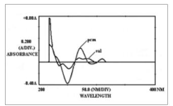
Fig. 3: Overlain second-order derivative spectrum of valdecoxib (val) and paracetamol (pcm) in methanol.
