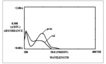
Fig. 1: Overlain spectra of valdecoxib (val) and paracetamol (pcm) in methanol.
