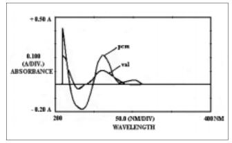
Fig. 2: Overlain first-order derivative spectrum of valdecoxib (val) and paracetamol (pcm) in methanol.
