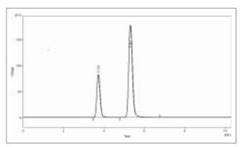
Fig. 1: HPLC chromatogram of venlafaxine hydrochloride (RT 3.7 min) and carbamazepine (RT 5.3 min).
