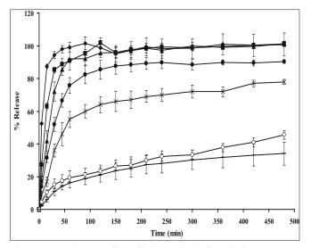
Fig. 1: Drug release profiles of indomethacin formulations Drug release profiles of indomethacin from tablets containing  $(-\bullet-)$  0% HPMC;  $(-\bullet-)$  5% HPMC;  $(-\bullet-)$  10% HPMC;  $(-\bullet-)$  15% HPMC;  $(-\times-)$  20% HPMC; (-O-) 25% HPMC and (---) capsules in phosphate buffer pH 6.2 (n=3).
