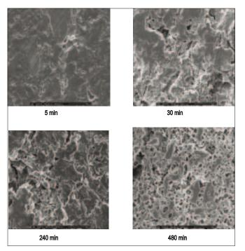
Fig. 7: SEM micrographs of tablets of 75 mg indomethacin. Scanning electron microscope micrographs of tablets containing 75 mg indomethacin and 25% HPMC in 70:30 PEG 4000:PEG 400 system after dissolution test in phosphate buffer pH 6.2 at different time interval with magnification of 250X.
