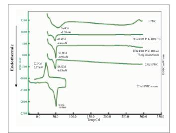
Fig. 5: DSC thermograms of HPMC and indomethacin tablets. Differential scanning calorimetric thermograms of HPMC, indomethacin tablet containing 25% HPMC in 70:30 PEG 4000:PEG 400 system and reverse run DSC study for indomethacin tablet containing 25% HPMC in 70:30 PEG 4000:PEG 400 system.
