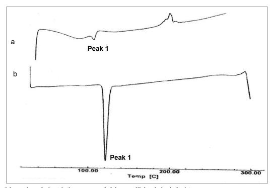
Fig 4: Differential scanning calorimetric thermograms of plain carvedilol and physical mixture. DSC thermograms of physical mixture of carvedilol with chitosan and conjugated chitosan (a, Peak onset was 111.90°, apex 115.17°, endset 119.39° and Heat change observed was -40.47 mJ) and plain carvedilol (b, Peak onset was 113.92°, apex 117.47°, endset 121.83° and Heat change observed was -339.97 mJ).
