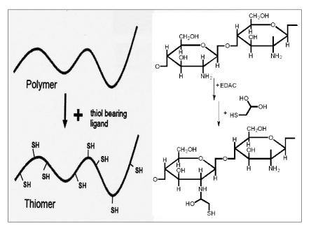
Fig 1: The presumptive substructure and synthetic pathway of chitosan-thioglycolic acid conjugates.
