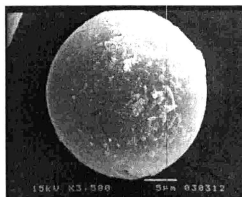
Fig. 2: SEM photomicrograph of ibuprofen-loaded polystyrene microspheres. SEM photomicrographs of a) showing spherical nature of polystyrene microspheres and b) showing the drug present on the surface of microspheres.
