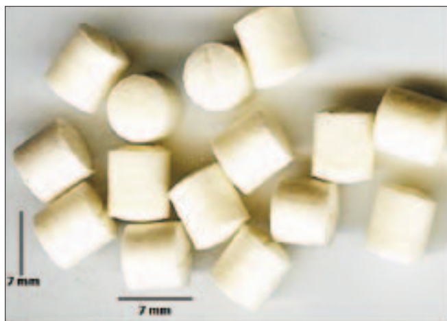
Fig. 1: Cefoperazone sodium impregnated calcium sulphate-polycaprolactone composite pellets
