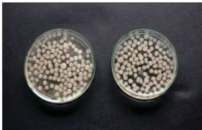
Fig. 1: Calcium alginate beads formed from 1-2 cm. These beads were obtained after sodium alginate addition from a height of 1-2 cm in to the CaCl 2 solution.
