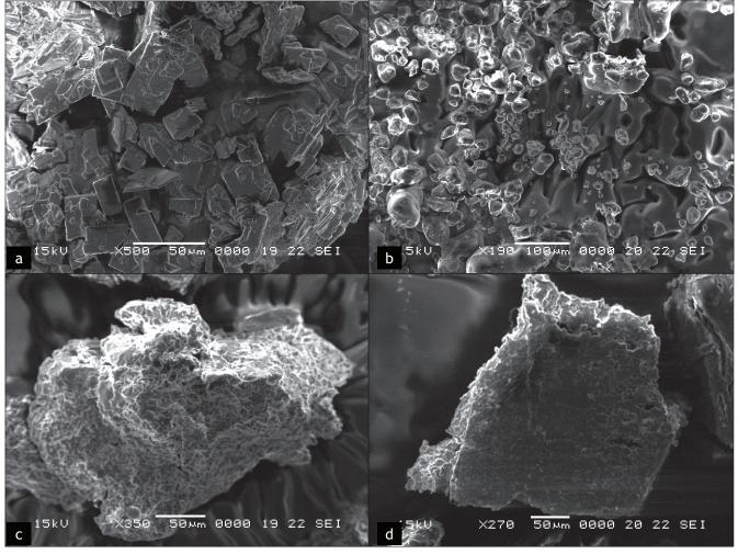
Fig. 1: Scanning electron micrography of aceclofenac and pharmacosomes (a) Aceclofenac, (b) Phospholipid, (c) Pharmacosome of aceclofenac 1:1(drug: lipid ratio) and (d) Pharmacosome of aceclofenac 2:1(drug: lipid ratio)
