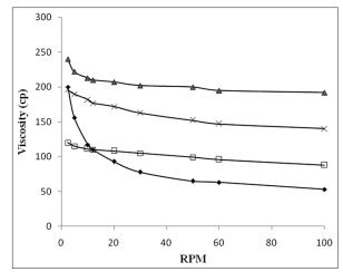
Fig. 1: Rheological behavior of the neat polymers. Pseudoplastic rheological behavior was observed with all the four polymers,  $(-\times-)$ sodium CMC 0.5%,  $(-\Box-)$  guar gum 0.5%,  $(-\bigstar-)$  xanthan gum 0.1% and  $(-\bigstar-)$  methyl cellulose 2%.
