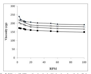
Fig. 5: Effect of  $\beta$ -CD on the rheological behavior of methyl cellulose. Decrease in viscosity was observed after addition of  $\beta$ -CD and as the proportion of cyclodextrin was increased, the viscosities decreased. (- $\phi$ -) methyl cellulose 2%,(- $\times$ -) methyl cellulose 2%+ $\beta$ -CD 0.5%, (- $\Delta$ -) methyl cellulose 2%+ $\beta$ -CD 1% and (- $\pi$ -) methyl cellulose 2%+ $\beta$ -CD 2%).
