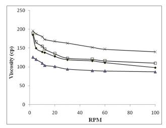
Fig. 4: Effect of  $\beta$ -CD on the rheological behavior of sodium CMC. Decrease in viscosity was observed after addition of  $\beta$ -CD and as the proportion of cyclodextrin was increased, the viscosities decreased, (-×-) sodium CMC 0.5%, (-□-) sodium CMC 0.5%+ $\beta$ -CD 0.5%, (- $\Box$ -) sodium CMC 0.5%+ $\beta$ -CD 2%).
