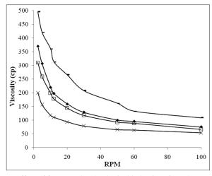
Fig. 2: Effect of  $\beta$ -CD on the rheological behavior of xanthan gum. Increase in viscosity was observed after addition of  $\beta$ -CD and as the proportion of cyclodextrin was increased, the viscosities also enhanced, (-×-) xanthan gum 0.1%, (-□-) xanthan gum 0.1%+ $\beta$ -CD 0.5%, (- $\diamond$ -) xanthan gum 0.1%+ $\beta$ -CD 1% and (---) xanthan gum 0.1%+ $\beta$ -CD 2%).
