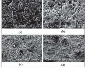
Fig. 7: SEM of tablet surfaces made by different methods SEM of tablet surfaces made from different methods (200X). (a) dry blend tablet, (b) spray dried blend tablet, (c) partial melt granulation tablet, (d) melt granulation tablet
