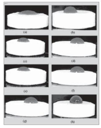
Fig. 6: Photoimages showing contact angle of water with tablet surfaces made by different methods before and after sintering Photoimages showing contact of water with tablet surfaces made from different methods before and after sintering. (a) Unsintered dry blending, (b) Sintered dry blending, (c) Unsintered spray drying, (d) Sintered spray drying, (e) Unsintered partial melt granulation, (f) Sintered partial melt granulation, (g) Unsintered melt granulation, (h) Sintered melt granulation.
