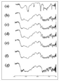
Fig. 9: FTIR of ketorolac tromethamine, Compritol® 888 ATO, physical mixture (control) and sintered tablets made from different methods
