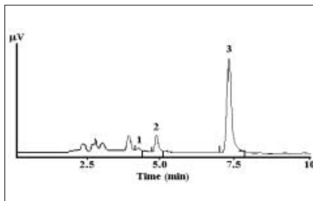
**Fig. 1: HPLC chromatogram of an incubation of p-nitrophenol with rabbit liver microsomes.** Incubations and HPLC analysis were performed as described in the text. The three peaks of interest are 1. Salicylamide (Internal standard, R.T. 4.26 min), 2. p-Nitrocatechol (R. T. 4.88 min), and 3. p-Nitrophenol (R. T. 7.35 min). HPLC chromatograms of the blank microsomes did not show presence of p-nitrocatechol peak.
