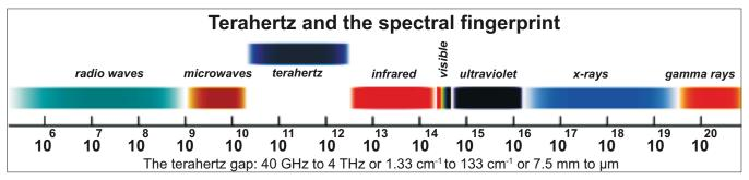
Fig. 1: electromagnetic spectrum of terahertz radiation (courtesy of SURA).
