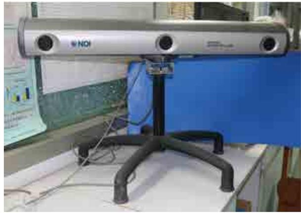
**Fig. 5: Optotrack motion measurement system**
